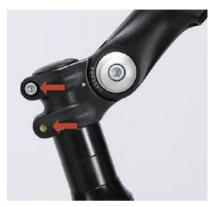
Loosen the bolt of adjustable stem, adjust the angle of stem inclination, and tighten the bolt of adjustable stem.
