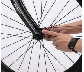
Squeeze the brake arms together and put brake noodle into the slot of noodle holder.
