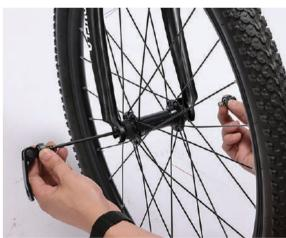
Turn the quick-release lever clockwise and tighten the wheel. Do not tighten too much since we need to lock the quick-release lever in the next step.
